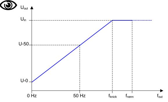
The diagram shows the relationship between output frequency ( $f_{out}$ ) and output voltage ( $U_{out}$ ). The position and steepness of the characteristic curve is determined by the two parameters U-0 (voltage when  $f_{out}$ =0Hz, also termed Boost) and U-50 (voltage when  $f_{out}$ =50Hz, can as a rule be taken from the motor rating plate).
