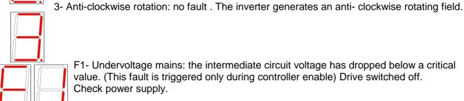
F1- Undervoltage mains: the intermediate circuit voltage has dropped below a critical value. (This fault is triggered only during controller enable) Drive switched off. Check power supply.
